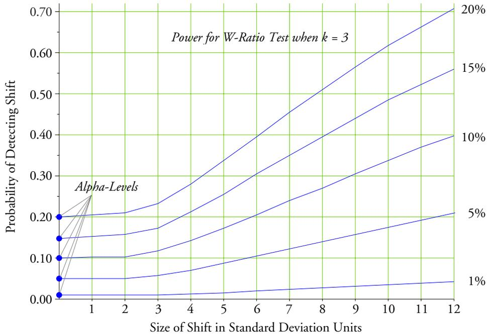
Figure 5: Power Functions for the  $W$ -Ratio Test when  $k = 3$  for Five Alpha-Levels
