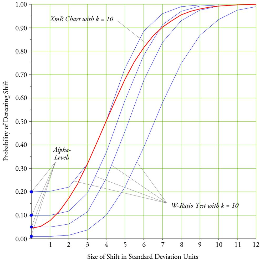
Figure 4: Why the *W*-Ratio Test Uses Alpha Levels of 10% to 20%
