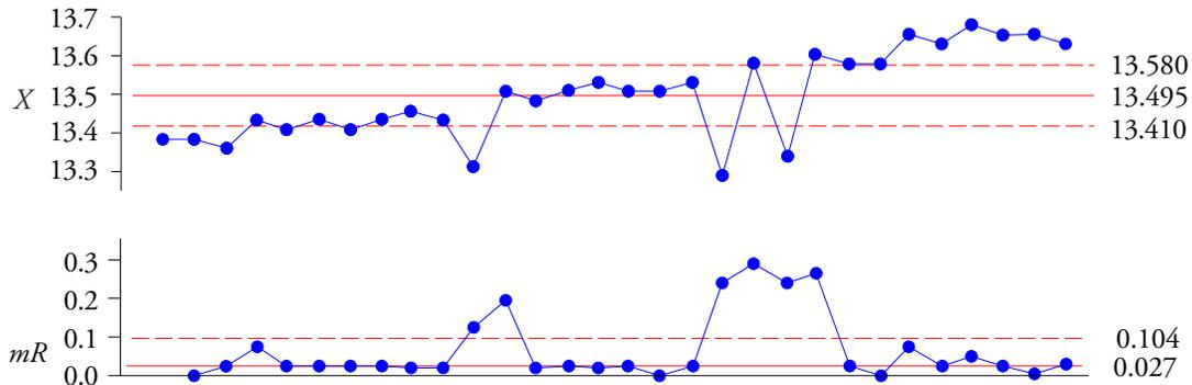
Figure 3: Consistency Chart for 30 Determinations of the Diameter of a Single Insert
